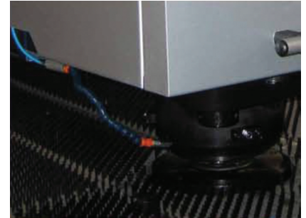
Punching Operation and Strip Lubrication
